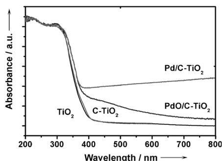
Figure 4. UV-visible absorption spectra of TiO<sub>2</sub> nanobelts, C-TiO<sub>2</sub> nanobelts, and PdO/C-TiO<sub>2</sub> and Pd/C-TiO<sub>2</sub> nanobelt heterostructures.
