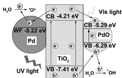
Figure 6. Illustration of the possible mechanisms of electron–hole separation and energy-band matching for PdO/C-TiO<sub>2</sub> and Pd/C-TiO<sub>2</sub> heterostructured nanobelts.
