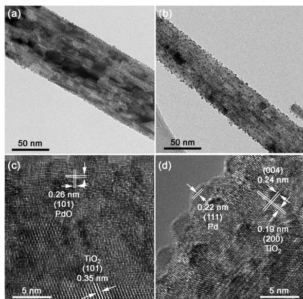
Figure 1. a, b) TEM images of C-TiO<sub>2</sub> nanobelts modified with PdO and Pd nanoparticles, respectively. c, d) The corresponding high-resolution TEM images of PdO/C-TiO<sub>2</sub> (2 wt %) and Pd/C-TiO<sub>2</sub> nanobelts.
