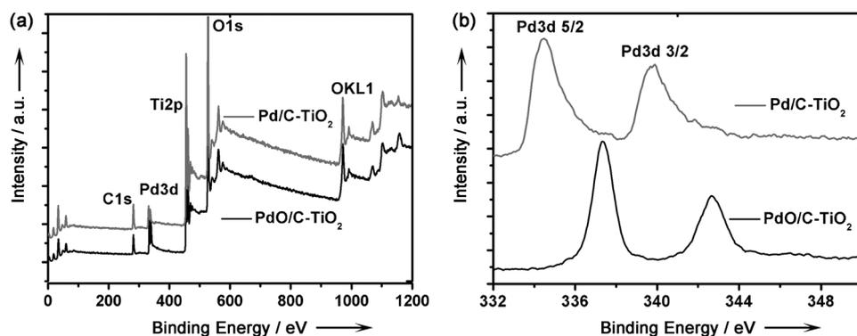
Figure 2. a) XPS survey spectra of PdO/C-TiO<sub>2</sub> and Pd/C-TiO<sub>2</sub> nanobelts. b) XPS spectra of the samples showing the Pd3d<sub>5/2</sub> and Pd3d<sub>3/2</sub> peaks.
