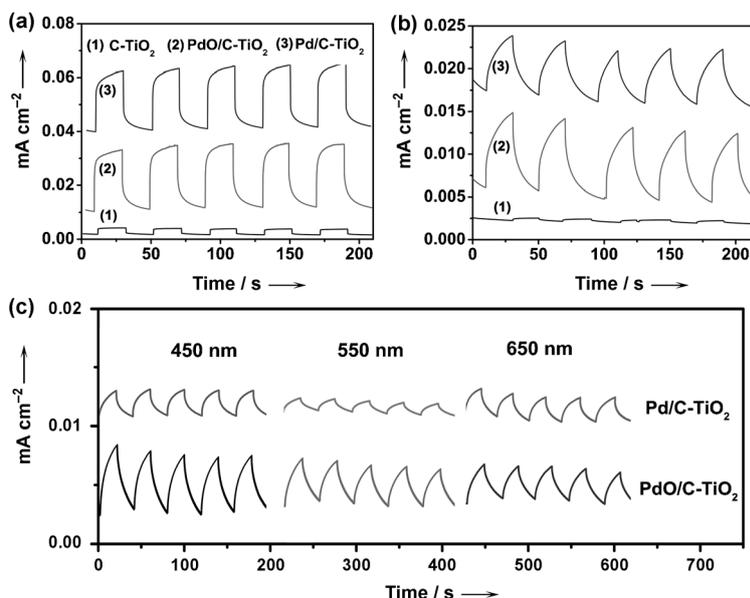
Figure 5. Time-dependent photocurrent response of the ITO photoelectrodes composed of C-TiO<sub>2</sub>, PdO/C-TiO<sub>2</sub>, and Pd/C-TiO<sub>2</sub>, respectively, at a bias voltage of 0.5 V. All the photocurrent intensities were normalized to the dark current. a) UV-light irradiation, b) visible-light irradiation, and c) monochromatic light irradiation at 450, 550, and 650 nm, respectively.
