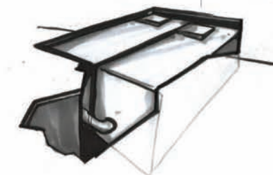
Underground Water Tank To pump water from canal and to store rainwater for research purpose.
