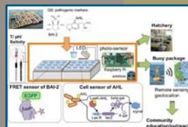
Paper-based sensors use plasmids to sense target and non-target quorum sensing molecules such as N-acyl homoserine lactones (AHLs) with detection by a shift from gray to blue on the paper and read-out by LED and photoresistors.
