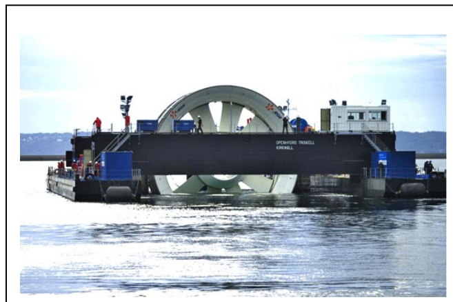
Fig. 11: A water current turbine, aimed at harnessing marine current energy, on its barge for transport and immersion offshore Paimpol (France).
