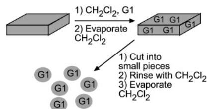
**Figure 1.** How the PDMS slabs were occluded with catalysts. A PDMS slab was swelled in CH<sub>2</sub>Cl<sub>2</sub> with the Grubbs' first generation catalyst. The Grubbs' catalyst diffused into the PDMS slab with CH<sub>2</sub>Cl<sub>2</sub>. The CH<sub>2</sub>Cl<sub>2</sub> was removed under vacuum and the PDMS slabs were briefly rinsed. The PDMS slabs were cut into mm-sized pieces and used in our reactions.
