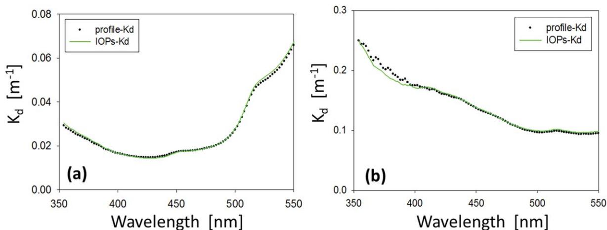
**Figure 2.** Examples showing remotely sensed  $K_d(\lambda)$  compared with profile  $K_d(\lambda)$  for (a) clear water (South Pacific Gyre) and (b) turbid water (Coast of Chile).
