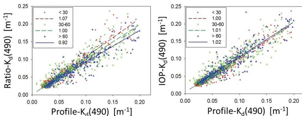
**Figure 7.** Comparison between retrieved  $K_d(490)$  and profile- $K_d(490)$  for various sun angle ranges of the NOMAD data set for  $K_d(490) < 0.2 \text{ m}^{-1}$ : (a) ratio-derived  $K_d(490)$  and (b) IOPs- $K_d(490)$ . The various regression lines are color coded and annotated with the regression slope values in the legend.
