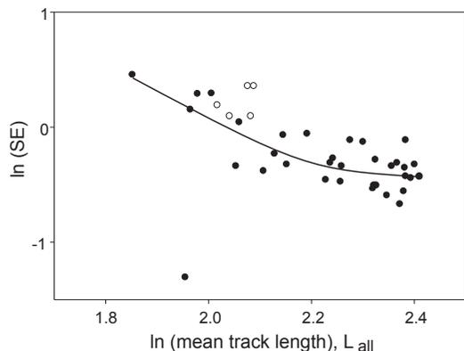
**FIGURE 4.** Empirically derived relationship between the mean track length and its standard deviation (SD), based on all annealing data from Tagami et al. (1998) (filled circles). For the proposed regression curve, the lowermost data point (in parentheses), which is based on only two measured track lengths, was neglected. Open circles show the standard error estimates that are visible in the figures of Kasuya and Naeser (1988).
