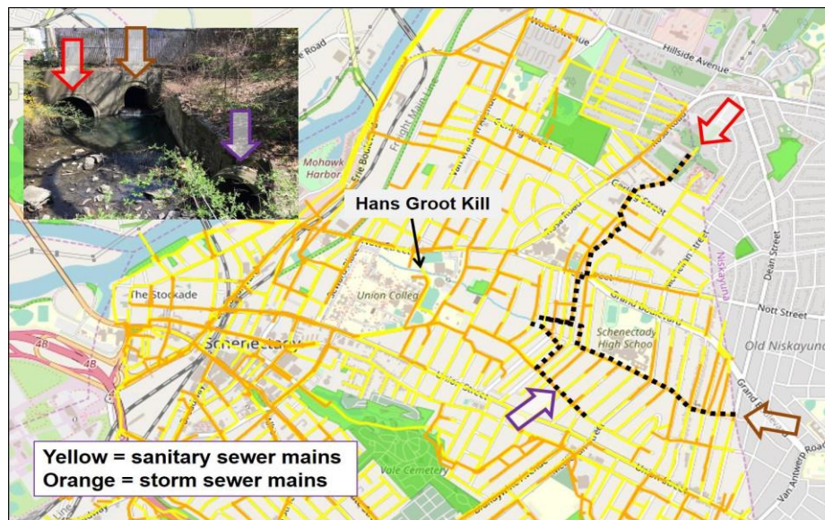
Figure 5: Base map provided by Schenectady County, using SIM GIS, shows storm and sanitary sewer mains. Dashed black lines indicate the three major storm sewer mains that provide the source water for the Hans Groot Kill. Inset photo shows the outfalls for the three storm sewer mains (red arrow = Sheridan Avenue, brown arrow = The Plaza, purple arrow = Rugby Avenue).
