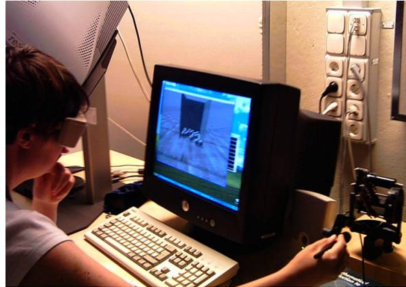
Figure 1: Interaction with the use of a PHANTOM.
