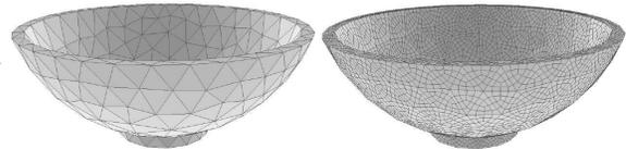
**Figure 4: Mesh of simulated bowl.**
