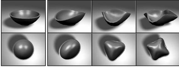
Figure 5: Simulated mode shapes of the bowl.
