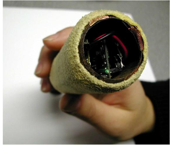
**Figure 1: The electronics inside the HyperPuja stick.**
