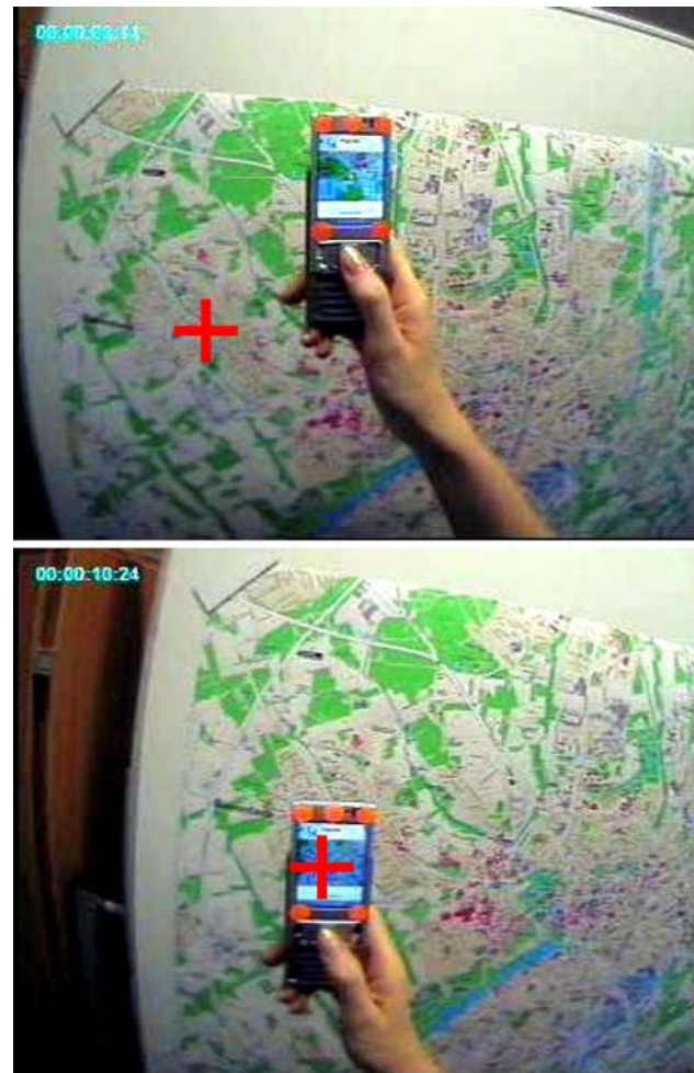
Fig. 6 Gaze—marked by the red eye tracking cursor—on the map (top) and on the handheld display (bottom). The figure shows two phases of movement towards the target. Gaze shift precedes hand movement (top) and hand follows to new gaze position (bottom)
