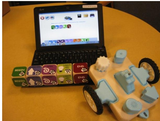
**Figure 4. The CHERP Tangible and Graphical Programming Interface**
