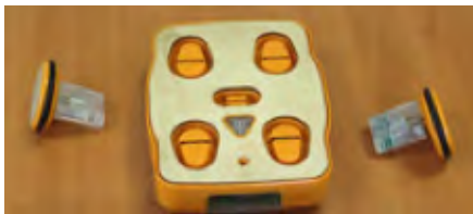
KIBO robot with wheels and motors
