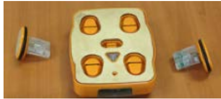
KIBO robot with wheels and motors
