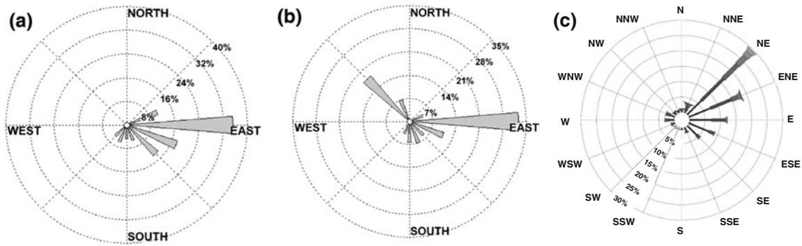
**Fig. 7** Directional wave distribution along the Spanish Coast. The radial axis indicates frequencies of occurrence. **a** Llobregat wave buoy that corresponds to the Barcelona coast, **b** Cap Tortosa buoy that
