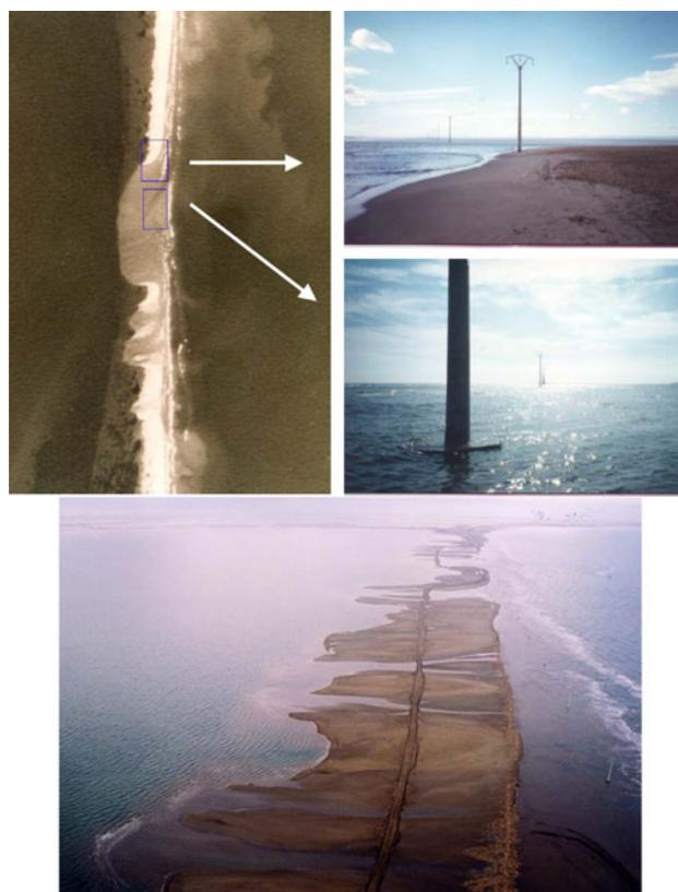
**Fig. 4** Storm impact in the Ebro region and, in particular, in the Trabucador Beach (*top-left*). Breaching after the impact of the October 1990 storm (*top-right*). Breaching after the November 2001 storm (*bottom*)
