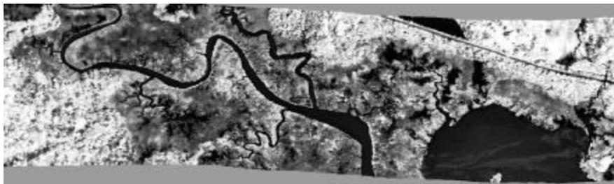
Fig. 6(a): The rule images of the linear spectral unmixing classification. It shows the oil appeared in Black surrounding the small streams on the river banks.
