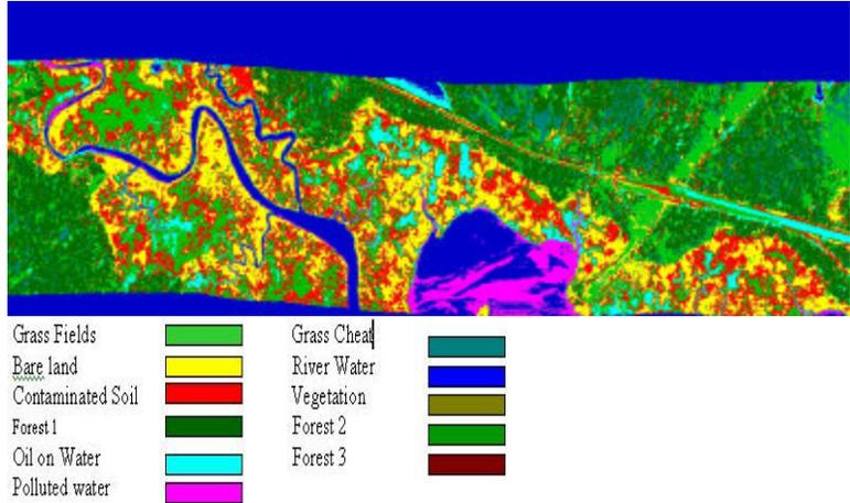
Fig. 5(b): supervised classification results. The contaminated soil with oil appeared in red and the oiled water on wetland appeared in cyan, the polluted water appeared in magenta.
