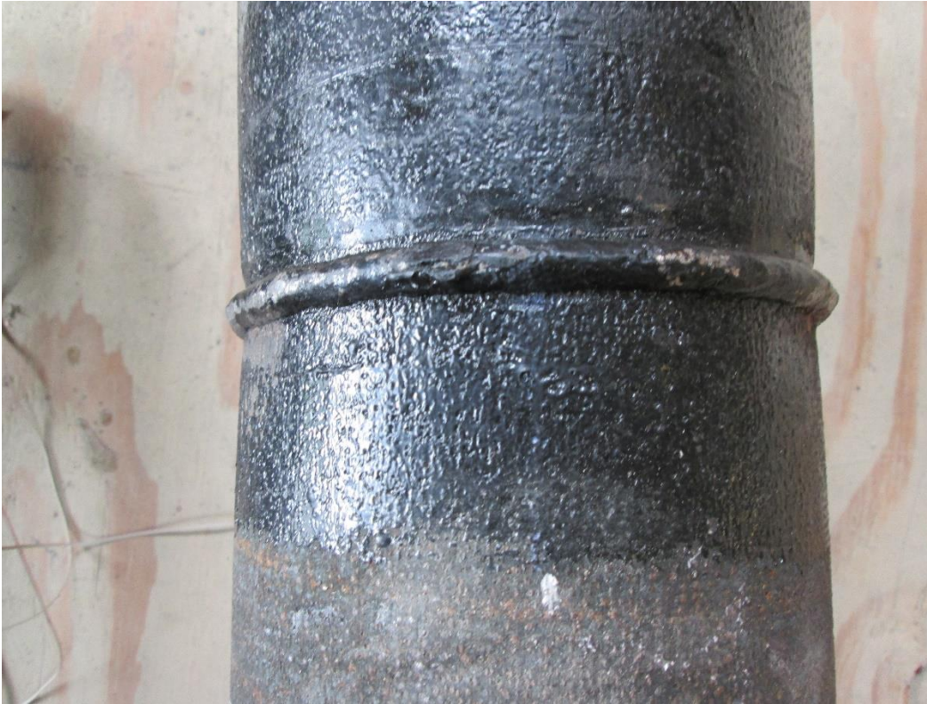
Figure 5.7. Deformed Area of the Spigot Caused by the Load Transferred from the Retaining Clips
