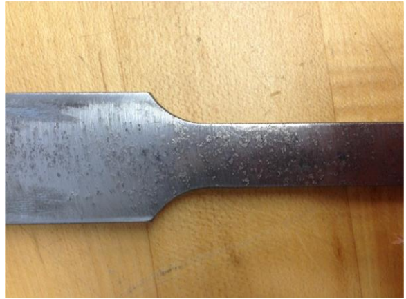
Figure 2.3. Surface Pitting on Ductile Iron Coupon before Machining of Reduced Area of Specimen 1
