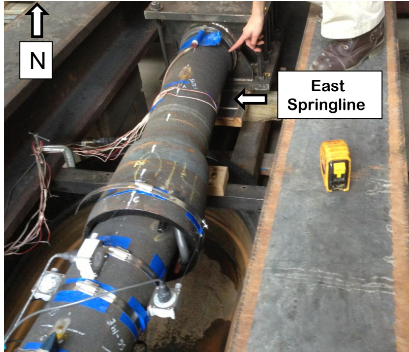
Figure 4.7. Photo of Compression Test on TR-Xtreme™ Joint
