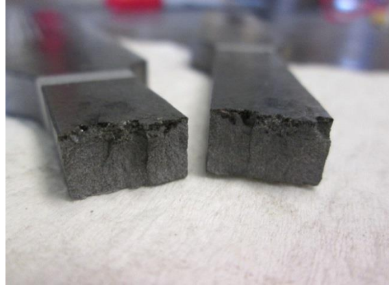
Figure 2.17. Fracture of Test Specimen 5 with Multiple Ridges
