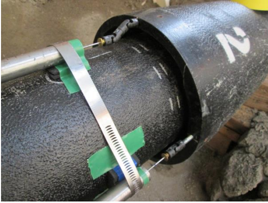
Figure 7.2 Setup of Springline DCDTs
