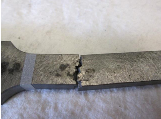
Figure 2.16. Uneven Fracture of Test Specimen 5
