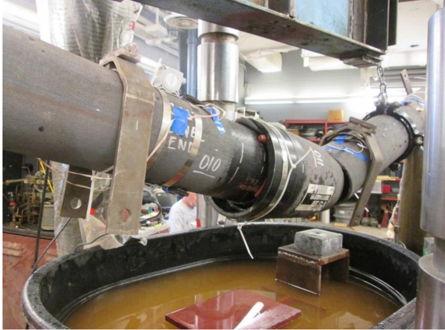
Figure 3.8. Pipe Failure in Test A
