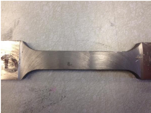
Figure 2.4. Surface of Ductile Iron Coupon after Machining of Reduced Area of Specimen 1
