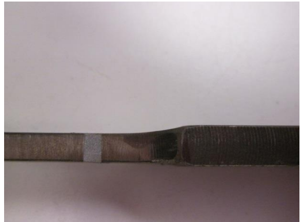
Figure 2.5. Machining of Surface to Reduce Surface Pitting on Specimen 1
