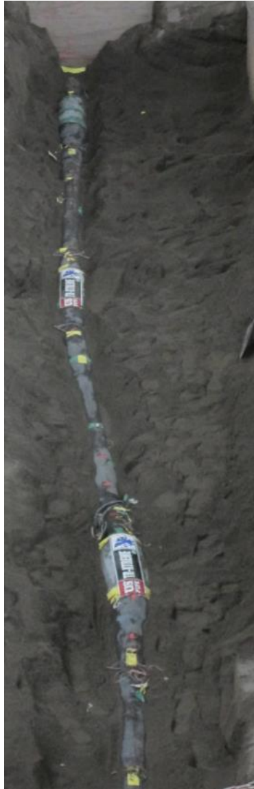
a) Deformed Pipe in Test Basin
