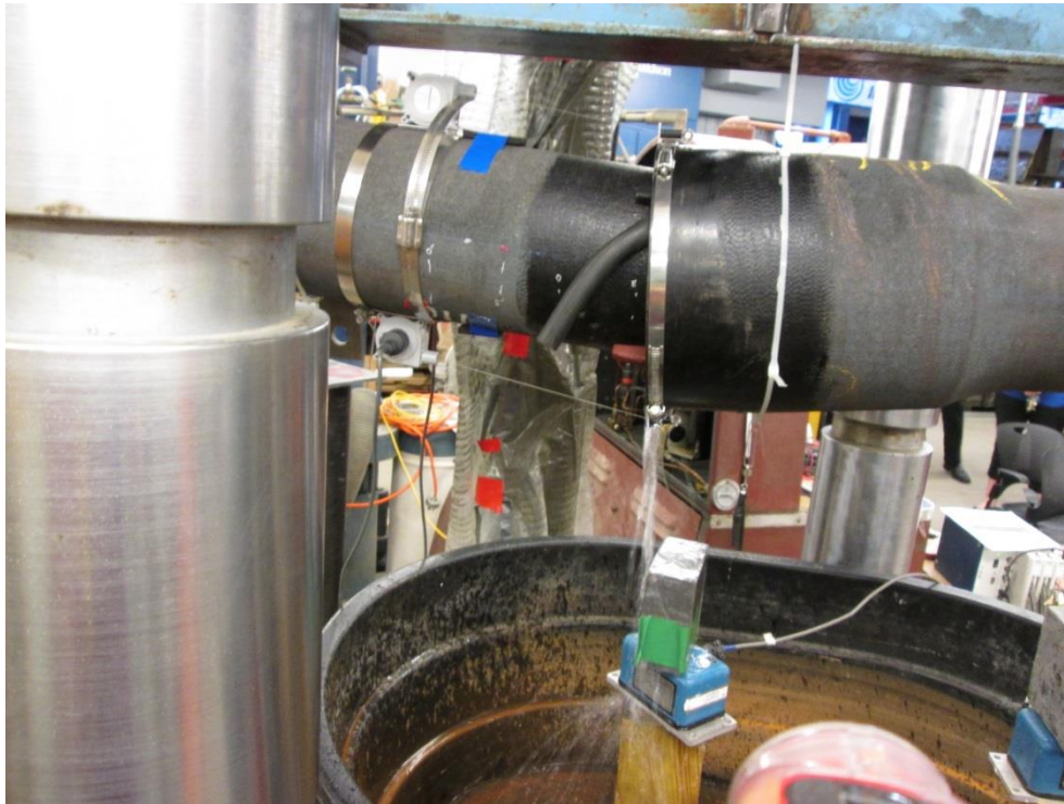
Figure 3.15. Leakage at Peak Moment in Test B
