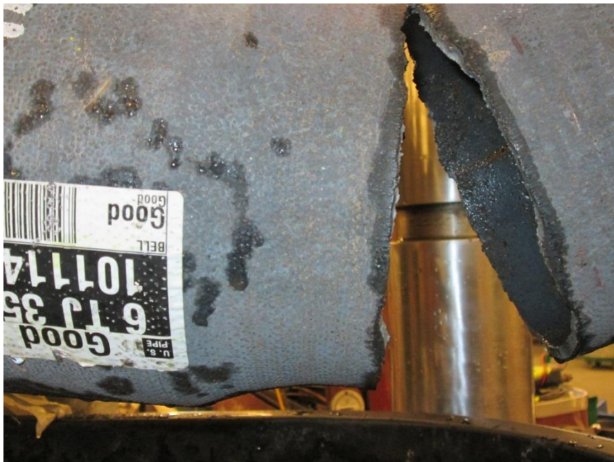
Figure 3.9. Side View of Pipe Failure in Test A
