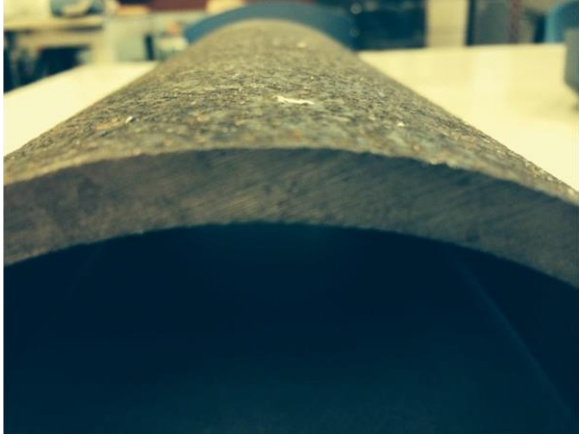
Figure 2.2. Ductile Iron Pipe Specimen with Significant Material Irregularities
