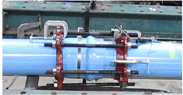
(b) Allowable Axial Displacement
