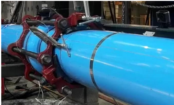
(c) Clamping Teeth Induce Pinching Effect
