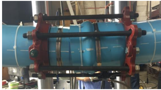
(b) Restrained Joint at 10 in. (254 mm.) of Displacement
