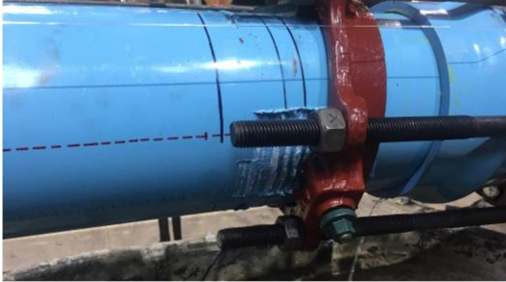
Figure 3.8. Fracture of Restraining Collar Clamping Tooth Housing
