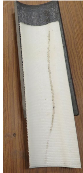
(b) View of Aqua-Pipe Lining and Pipe Specimen after Being Cut and Prepared
