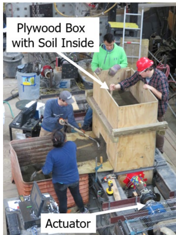
Figure 6.4. Soil Box Used in Direct Compression Tests
