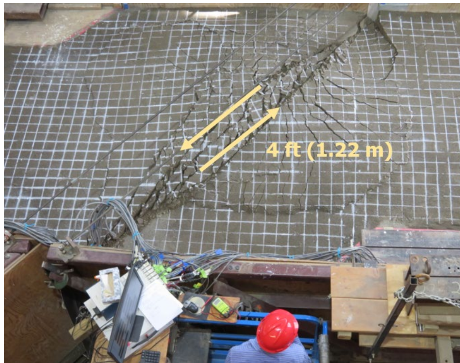
Figure 9.23. Maximum Fault Rupture
