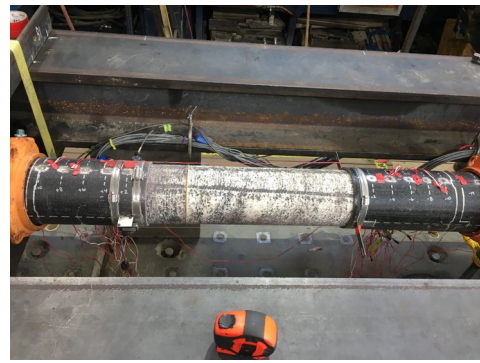
(d) View of Lining Exposed After Completion of Actuator Displacement
