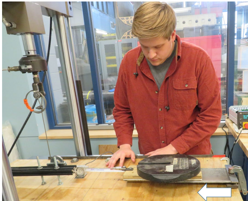
Figure 5.2. Photo of Aqua-Pipe Direct Shear Test Setup
