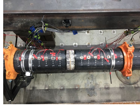
(b) View of Lining Exposed After First 6 in. (152 mm) of Actuator Displacement
