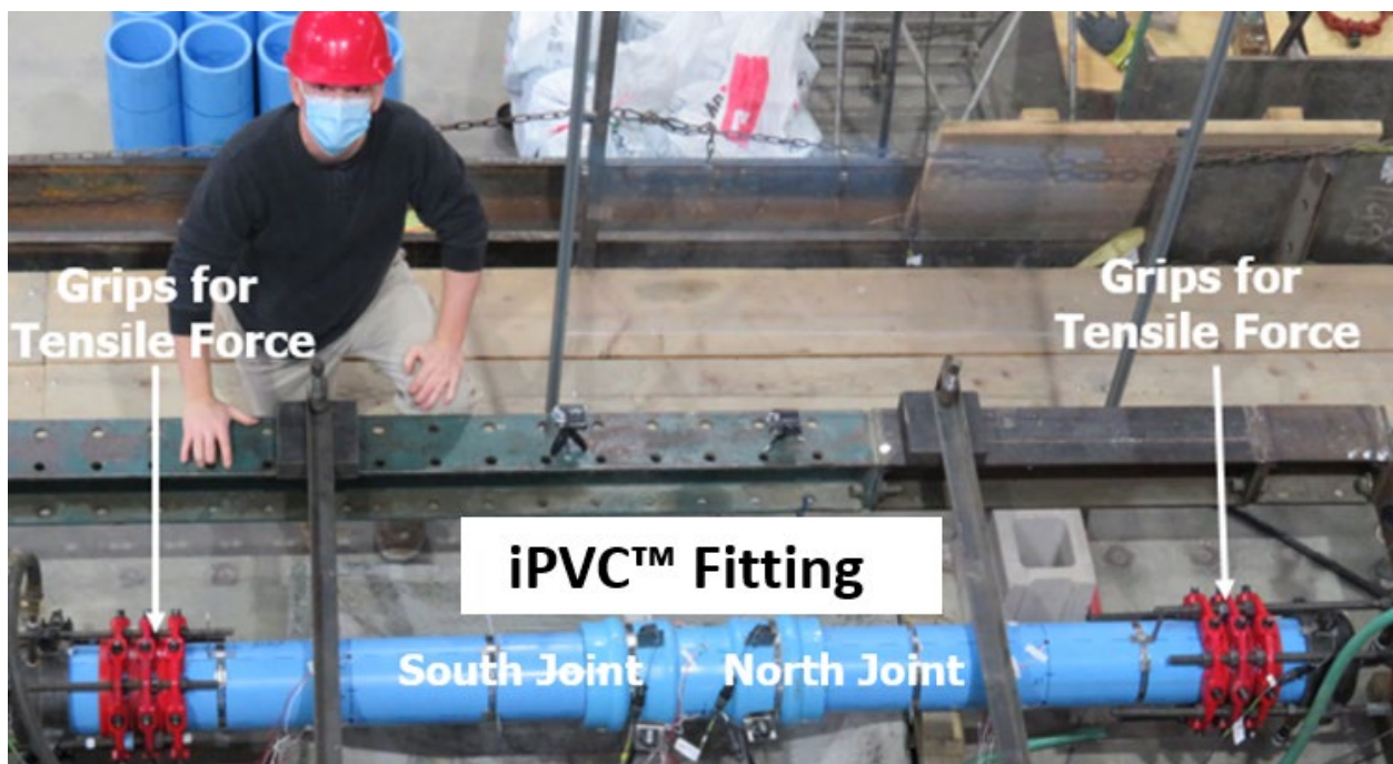
Figure 3.2. Test Specimen in the Direct Tension Frame
