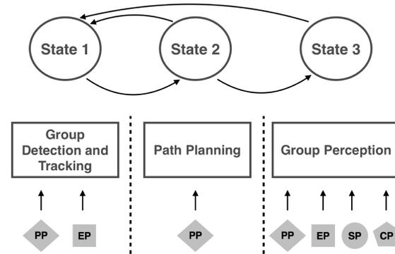
**Figure 1: Affiliation System.** State 1 is designed based on the PP and EP; therefore, it detects and tracks groups of people. State 2 plans a path trajectory from the robot's current position to a goal position in a group, which is designed based on the PP. State 3 allows the robot to perceive the affiliative state of groups using all four principles of attraction.
