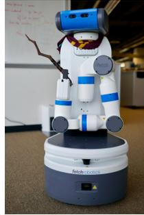
**Figure 2:** We use the Fetch in our work which stands at human height and is equipped with an RGB-D sensor, back-drivable 7-DOF arm, and a 2D laser scanner.
