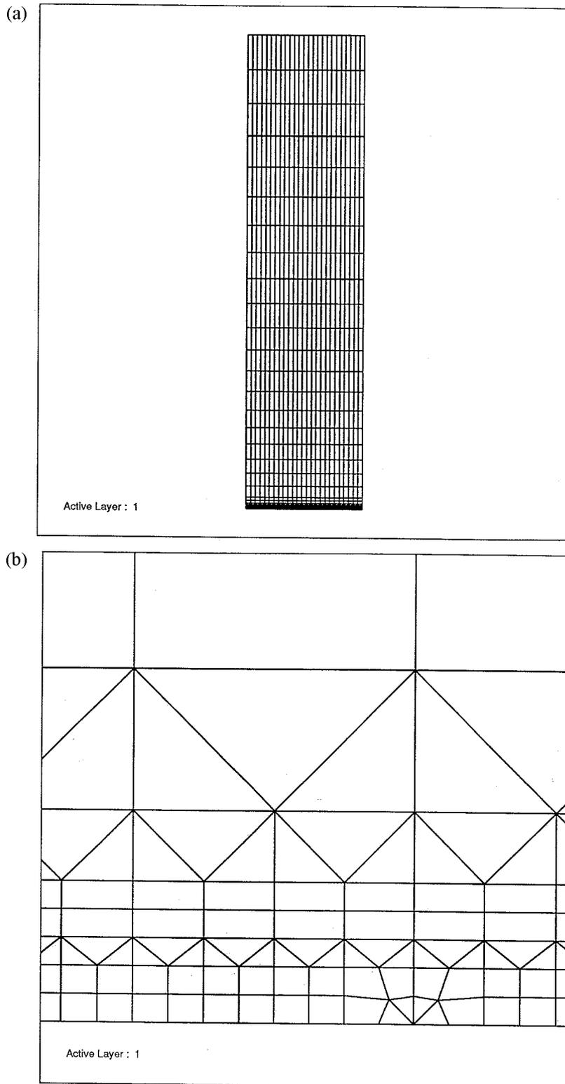
Figure 5. (a) Mesh used for layered finite element analysis. (b) Detail of the mesh near the crack tip.
