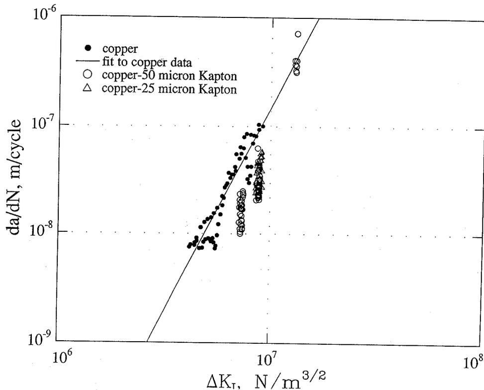
Figure 10. Fatigue crack growth rate for copper and copper-polyimide samples,  $R = 0.2$ . Note that although the copper-polyimide data fall close to the copper data, the loads for the copper-polyimide samples were much higher than for the copper samples. The stress intensity factors, however, are approximately the same due to the large amount of crack tip shielding provided by the polyimide.
