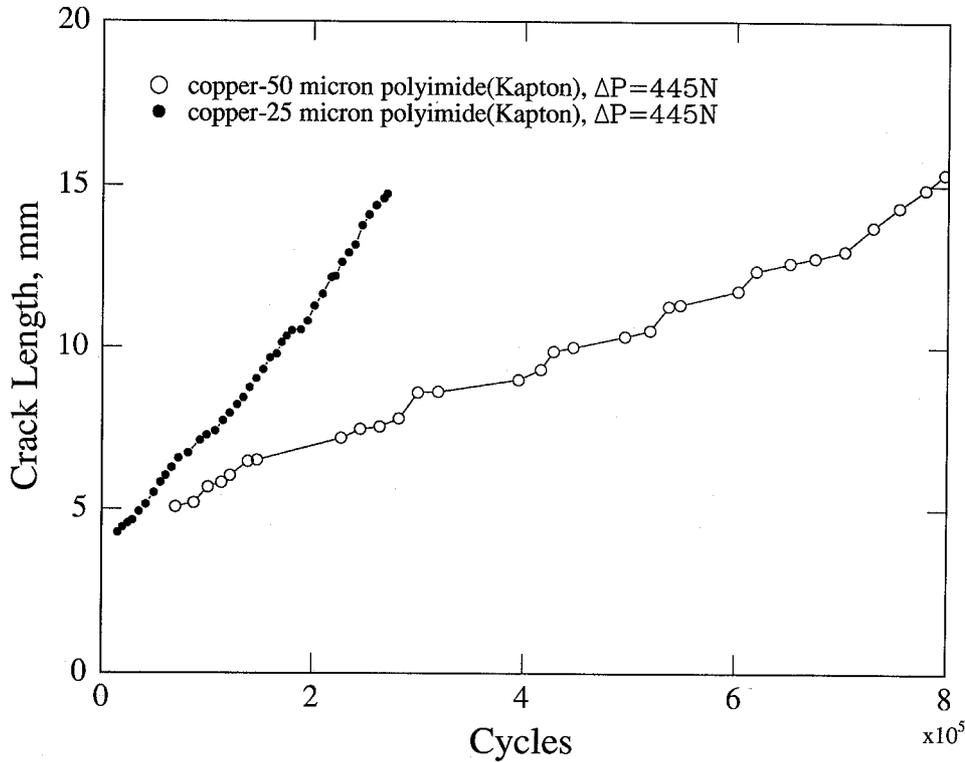
Figure 11. Crack length record for laminates with 25  $\mu\text{m}$  and a 50  $\mu\text{m}$  polyimide. Both tests were run at  $\Delta P = 445\text{N}$ . The rate of crack growth in the 25  $\mu\text{m}$  polyimide laminate is approximately three times faster than in the 50  $\mu\text{m}$  laminate.
