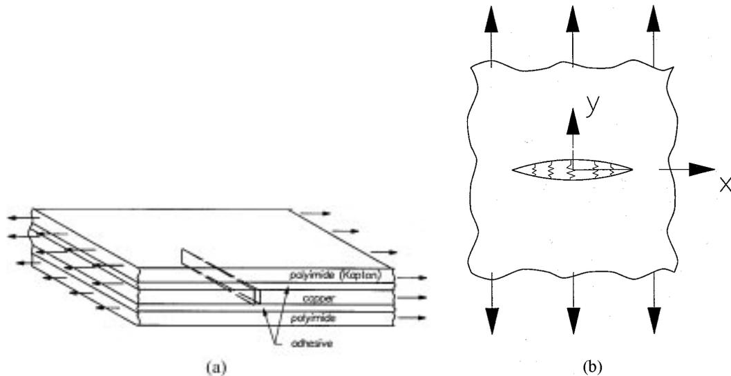
Figure 1. (a) Crack growth in copper, note that the polyimide layers remain intact. (b) Idealization of the polyimide layers bridging the crack as linear springs.
