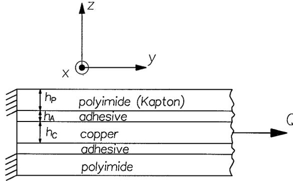
Figure 2. Layup of laminates, and geometry for shear lag model. View is of a cross section perpendicular to the crack line. Tensile stress in the laminate away from the crack is carried across the crack by the intact polyimide layer.
