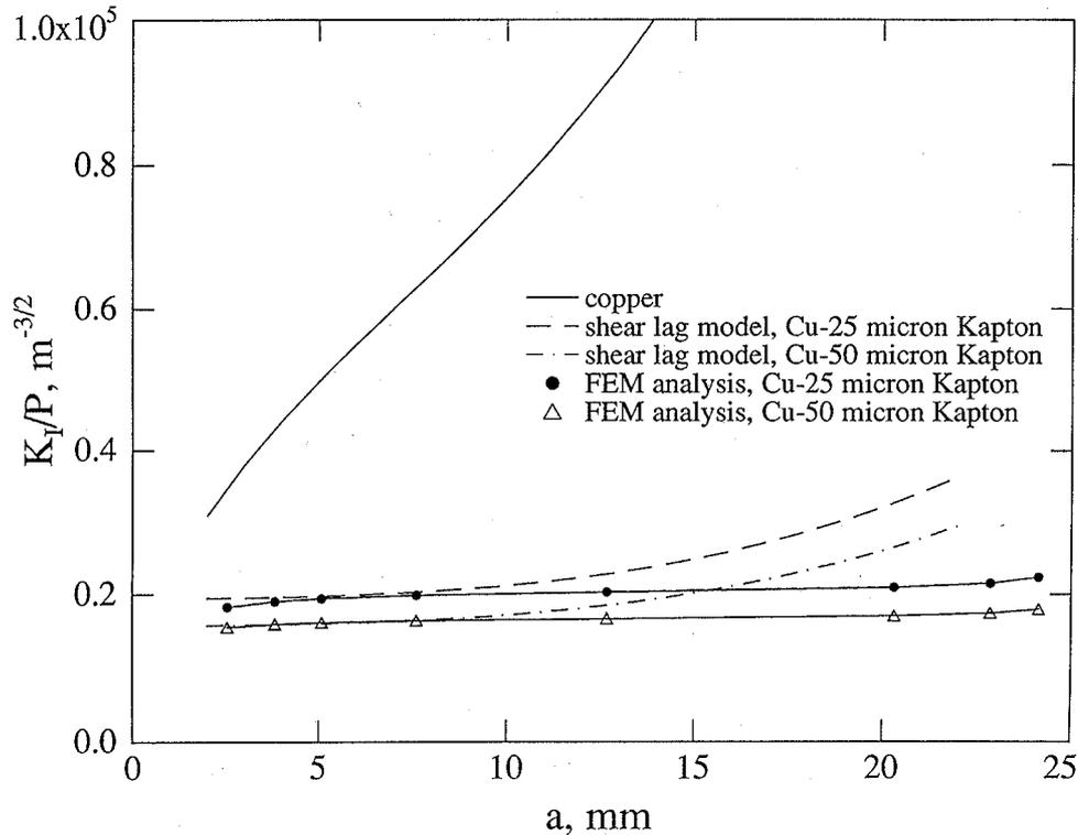
Figure 4. Stress intensity factor vs. crack length for the pure copper sample, and for the copper-polyimide samples analyzed using the shear lag and finite element models.
