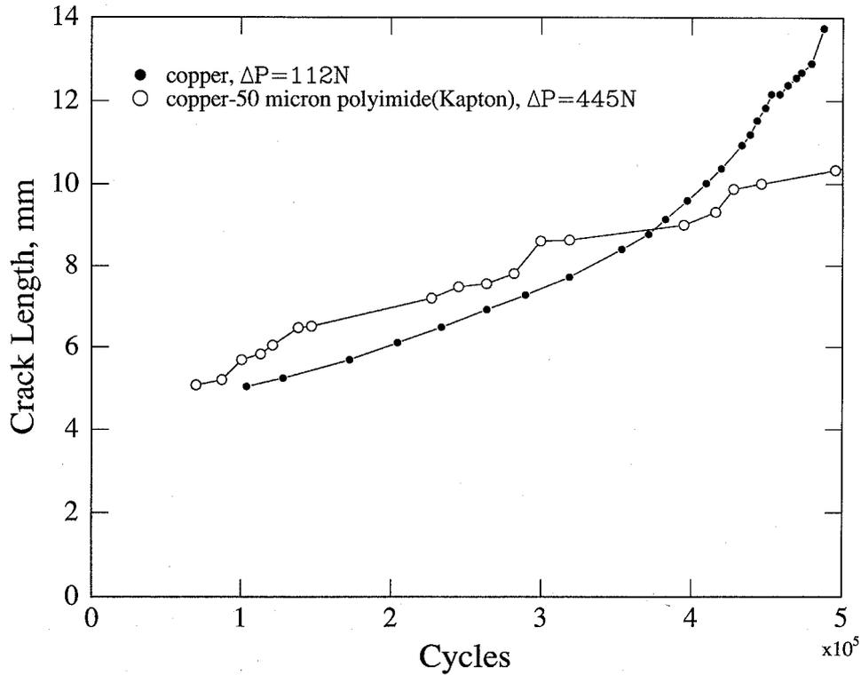
Figure 9. Crack length record for a pure copper sample loaded at  $\Delta P = 112N$ , and for a copper-polyimide sample loaded with  $\Delta P = 445N$ .
