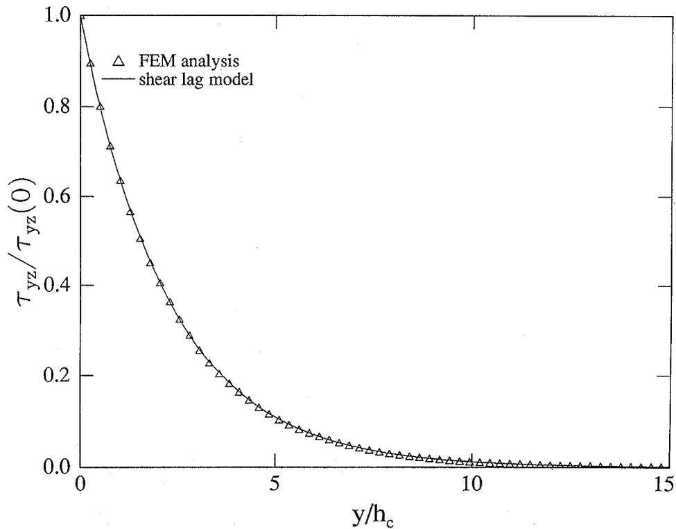
Figure 7. Shear stress distribution normal to the crack line. Results are for 50.8  $\mu m$  thick polyimide.
