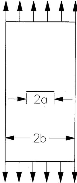
Figure 3. Center cracked test specimen.  $2b = 50.8$  mm. Length = 208 mm.
