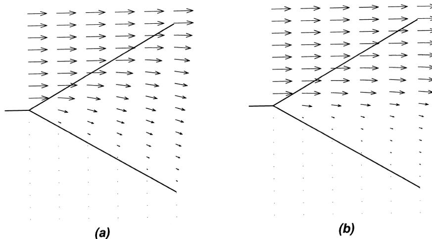
Fig. 2. (a) Velocity vectors for the symmetric, linear  $v_x$  field. (b) Velocity vectors for symmetric, non-linear  $v_x$  field with  $s = 3$ .
