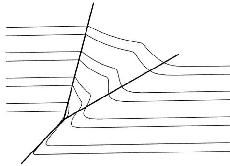
Fig. 6. Deformation resulting from asymmetric linear field using  $\tan \varphi_2 = 1/2 \tan \varphi_1$ ,  $\varphi_1 = 30^\circ$ , and placing one kink along  $y = 0$ .
