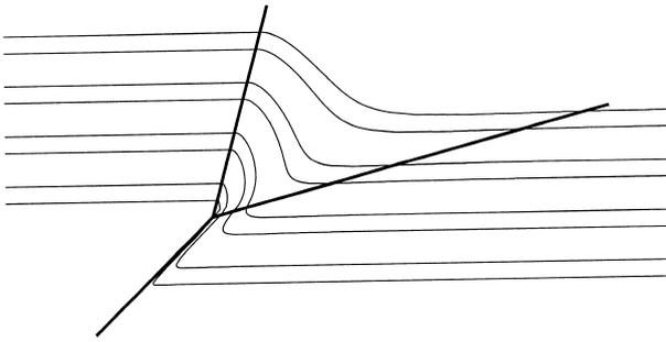
Fig. 5. Deformation resulting from sine field. Note that, even though  $P/S = 1$ , no sharp kink occurs at the hanging wall boundary of the trishear zone even though this boundary is fixed in the material.
