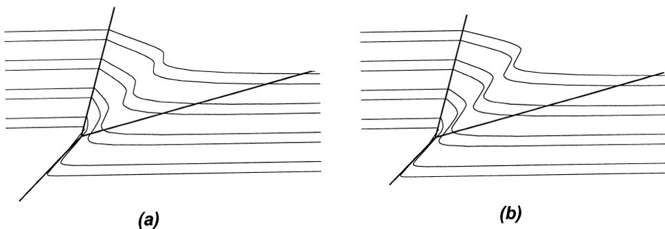
Fig. 4. Deformation resulting from non-linear field, (a)  $s = 2$ , (b)  $s = 3$ . As  $s$  increases, deformation concentrates towards center of the trishear zone.
