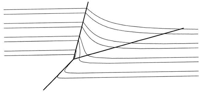
Fig. 3. Deformation resulting from linear field,  $s = 1$ . Thin lines are bedding tops and thick lines are the fault and the trishear zone boundaries. In all of the plots, Figs. 3–6,  $(P/S)=1$ , ramp angle =  $45^\circ$ . Trishear angle,  $2\varphi = 60^\circ$  for Figs. 3–5.
