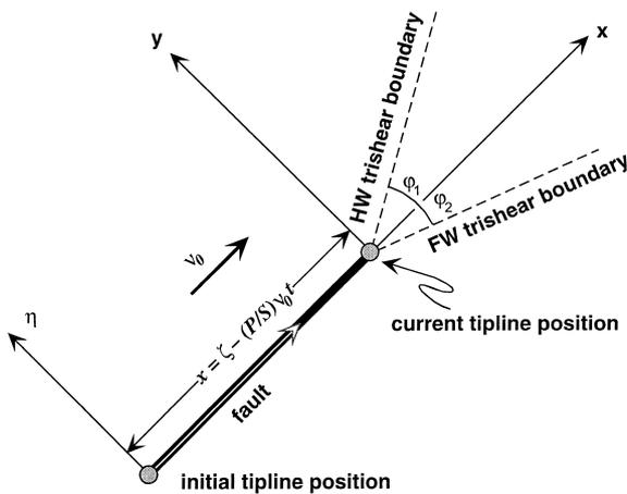
Fig. 1. Geometry of the trishear model showing co-ordinate systems used in the text. Note that the apical angle of the hanging wall and footwall trishear boundaries need not be the same. See text for definition of symbols.
