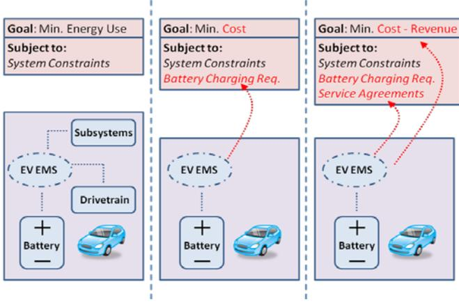
Fig 2. EV prosumer interactions. a) Standalone mode, b) Passive mode (provides charging constraint only), c) Multi-service mode (prosumer may provide energy and ancillary services).
