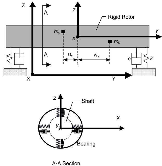
FIGURE 1. GEOMETRIC SETUP OF THE RIGID ROTOR.
