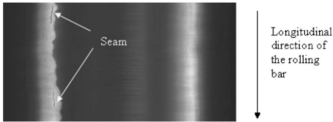
Fig. 1 A portion of a sensing image from a bar-rolling process
