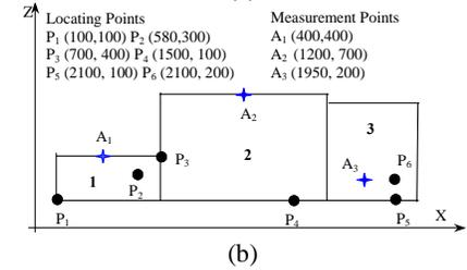
Figure 9. Geometry of the assembly
