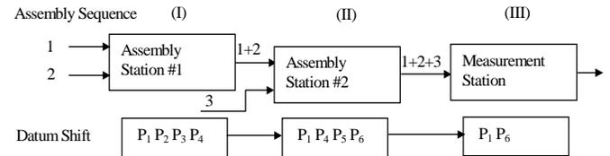
Figure 10. Assembly sequence and datum shift
