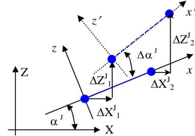
**Figure 6. Deviation of the local coordinate system**
