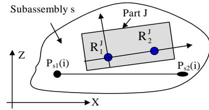
Figure 8. Fixture error-induced deviation
