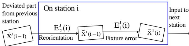
Figure 7. Deviation accumulation of part J on station  $i$
