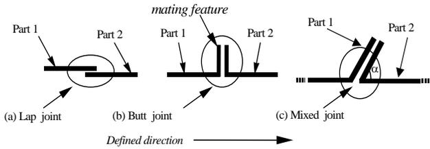
Figure 2. Cross-sectional views of joint geometries
