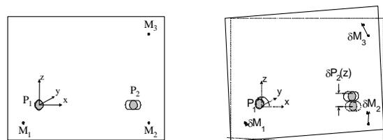
(a) Locators and measurements (b) Manifestation of  $P_2$  failure
