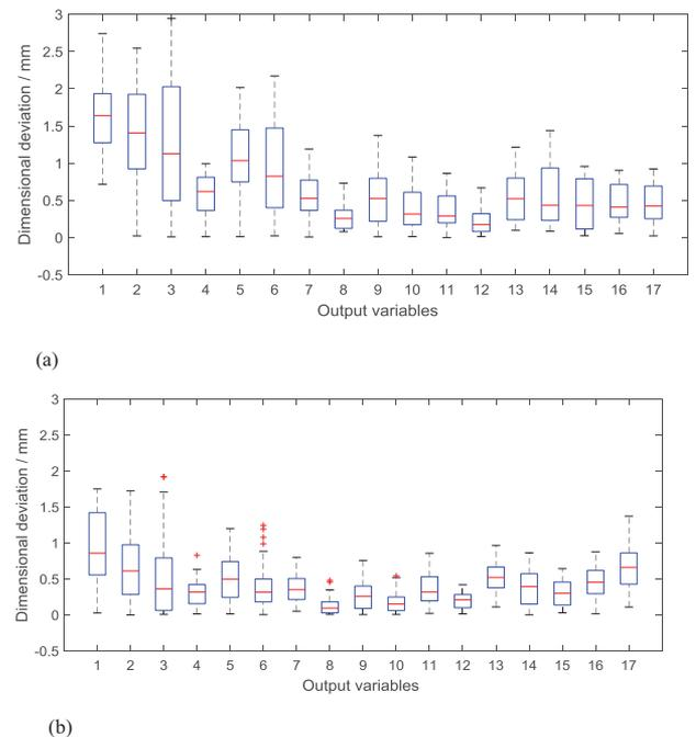
**Figure 8.** Prediction results of composite parts' assembly processes with or without optimal feed-forward control: (a) box plot of dimensional deviations without optimal feed-forward control; (b) box plot of dimensional deviations with optimal feed-forward control.
