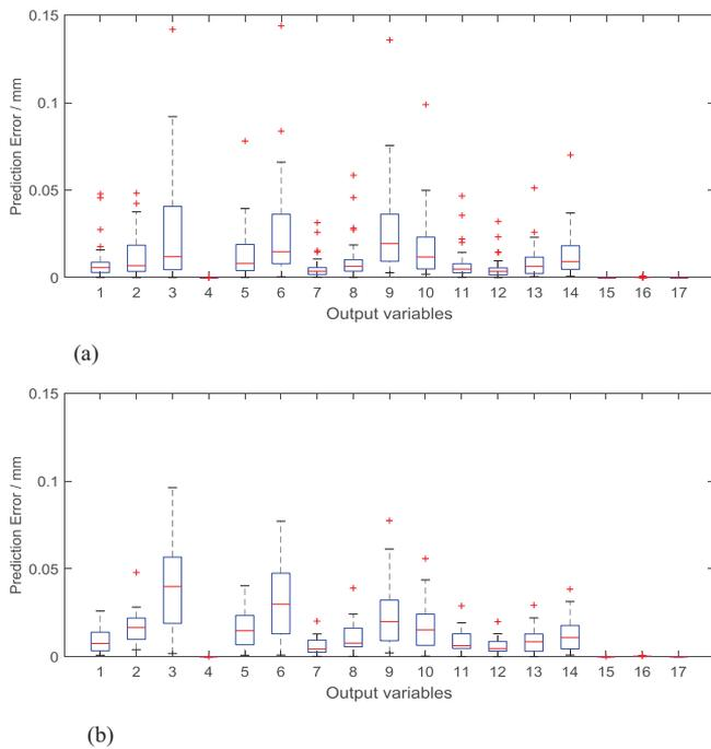
**Figure 7.** Prediction error of the universal Kriging model with or without optimal feed-forward control: (a) prediction errors without optimal feed-forward control; (b) prediction errors with optimal feed-forward control.
