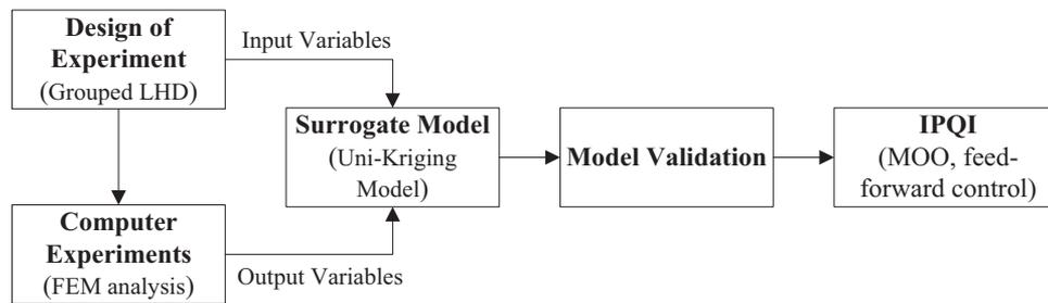
**Figure 1.** An overview of the proposed surrogate model-based feed-forward control.
