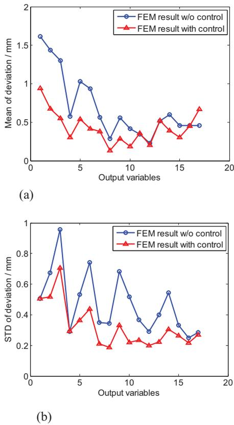
**Figure 9.** FEM results of composites' assembly processes with or without optimal feed-forward control: (a) mean of dimensional deviations; (b) STD of dimensional deviations.
