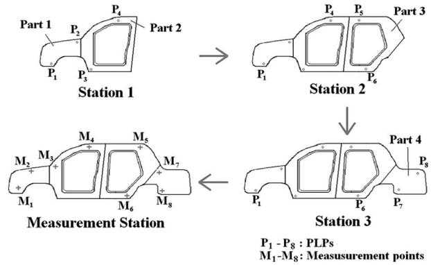
Fig. 7 Assembly sequence of a sedan side frame
