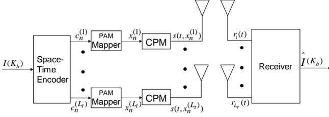
Fig. 1. Space-time coded CPM system.
