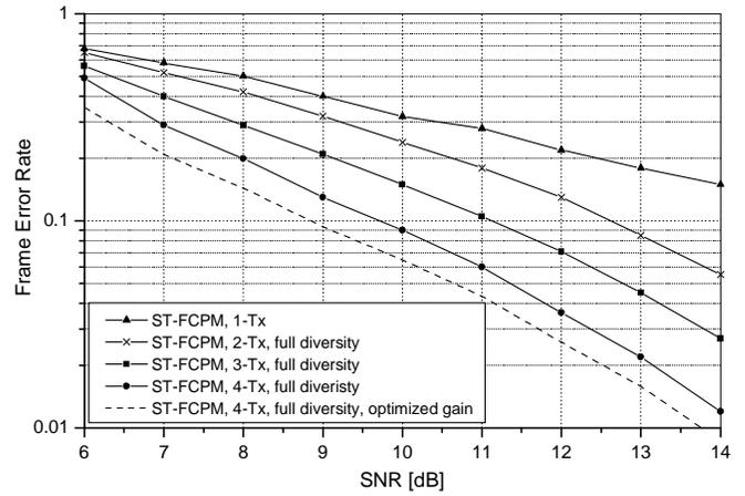
Fig. 2. Frame-error rate of 8-ary ST-CPM with IRC and  $h = 1/4$  in quasi-static fading.
