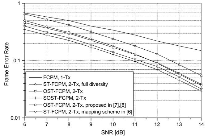
Fig. 3. Frame-error rate of  $(2 \times 2)$  8-ary ST-CPM with IRC and  $h = 1/4$  in quasi-static fading.
