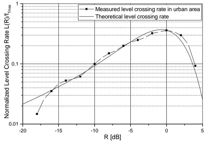
Fig. 7. The theoretical and the measured LCR in an urban surface street area.
