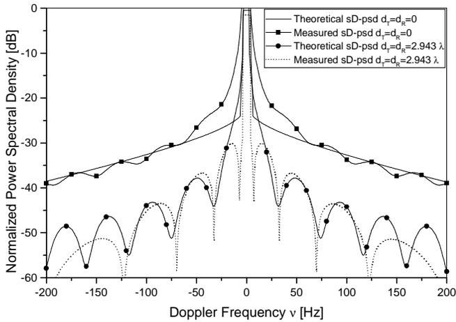
Fig. 5. The theoretical and the measured sD-psd in an urban surface street area.
