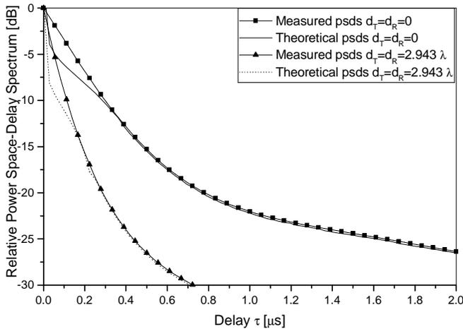
Fig. 6. The theoretical and the measured psds in an urban surface street area.
