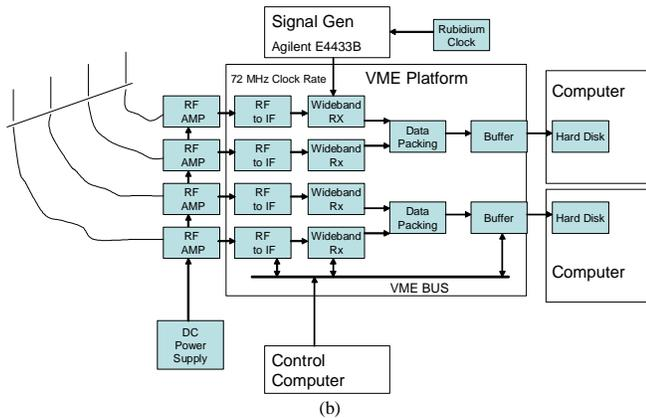
Fig. 2. The block diagram of the MIMO transmitter system (a) and the block diagram of the MIMO receiver system (b).
