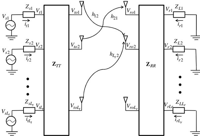
Fig. 1. Modeling of a MIMO V-to-V system using z- and h-parameters.
