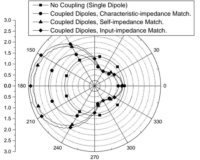
Fig. 3. The coupled dipole antenna patterns in the azimuthal plane, terminated with the characteristic, self-, and input-impedance matching network.
