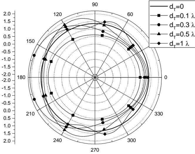
Fig. 2. The coupled dipole antenna pattern in the azimuthal plane as a function of antenna element spacings. The second dipole antenna is terminated with  $Z_c = 50\Omega$ .
