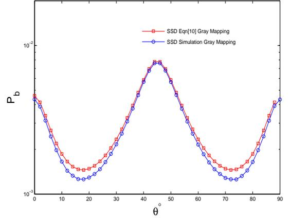
Fig. 4. Average probability of error  $P_b$  and  $P_b^{UB}$  versus rotational angle  $\theta$  of an SSD system using QPSK signal constellation over Rayleigh fading channel with perfect CSI at  $E_b/N_0 = 15$  dB. Gray signal constellation mapping is used.
