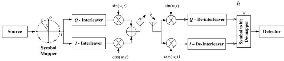
Fig. 1. System model (referred to as SSD system).
