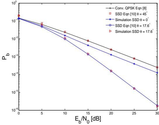
Fig. 3. Average probability of error  $P_b$  of conventional and SSD systems using QPSK signal constellation over Rayleigh fading channels with perfect CSI. Gray signal constellation mapping is used.
