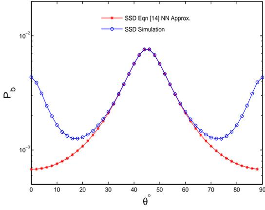
Fig. 2. Average probability of error  $P_b$  and  $P_b^{NN}$  versus rotational angle  $\theta$  of an SSD system using QPSK signal constellation over Rayleigh fading channel with perfect CSI at  $E_b/N_0 = 15$  dB. Gray signal constellation mapping is used.
