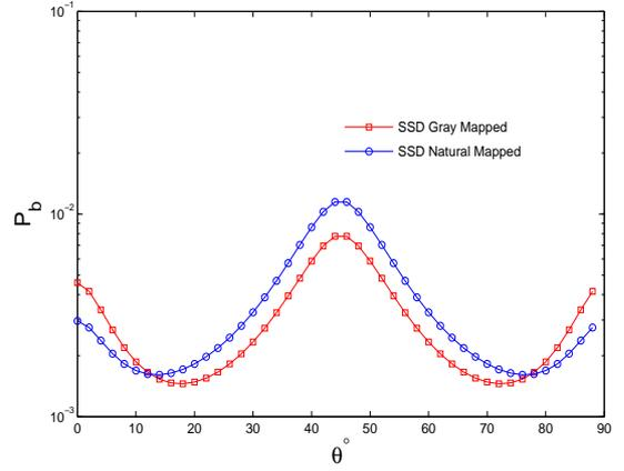
Fig. 5. Average probability of error  $P_b$  for Gray and Natural mapped QPSK signal constellation over Rayleigh fading channel with perfect CSI at  $E_b/N_0 = 15$  dB.
