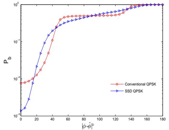
Fig. 6. The effect of phase estimation error on the performance of an SSD system ( $\theta = 22.5^\circ$ ) with respect to a conventional QPSK system at  $E_b/N_0 = 15$  dB. At the receiver coherent detection is carried out. Gray signal constellation mapping is employed.
