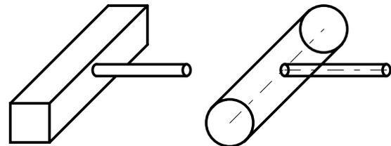
Figure 2. Exact dynamic three-dimensional model and thin-wire model of a boom and attached dipole arm.
