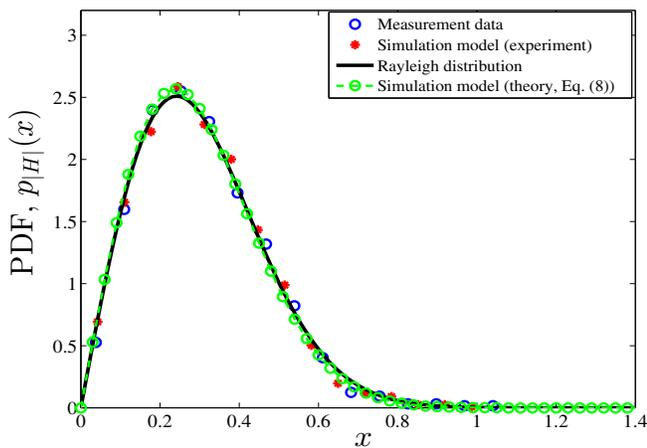
Fig. 7. The PDF of the UWA channel envelope .
