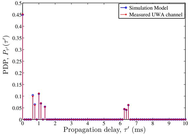
Fig. 6. The PDP  $\check{p}_{\tau'}(\tau')$  of the UWA measured channel compared to the PDP  $\bar{p}_{\tau'}(\tau')$  of the simulation model.
