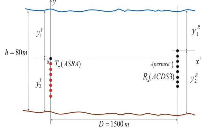
Fig. 1. The measurement configuration of the experiment for SIMO fixed-to-fixed (F2F) communication.
