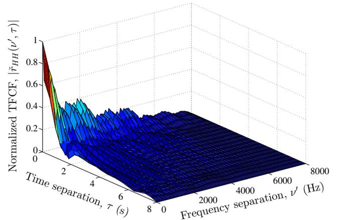
Fig. 4. Absolute value of the normalized TFCF  $|\tilde{r}_{HH}(\nu', \tau)|$  of the measured UWA channel.
