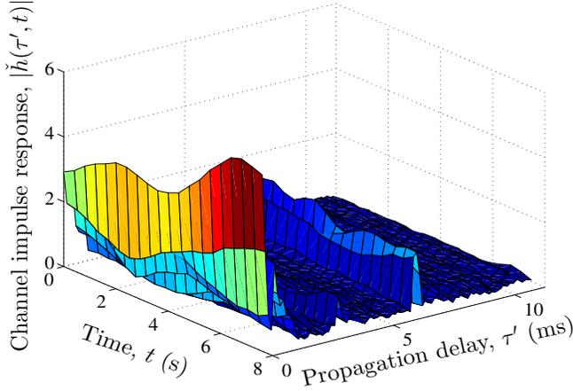
Fig. 2. Absolute value of the TVCIR  $|\hat{h}(\tau', t)|$  of the measured UWA channel.
