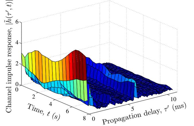
Fig. 3. Absolute value of the TVCIR  $|\hat{h}(\tau', t)|$  of the simulation model.
