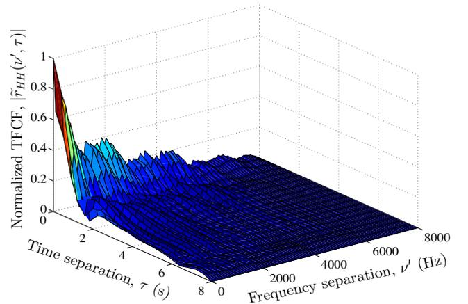
Fig. 5. Absolute value of the normalized TFCF  $|\tilde{r}_{HH}(\nu', \tau)|$  of the simulation model.
