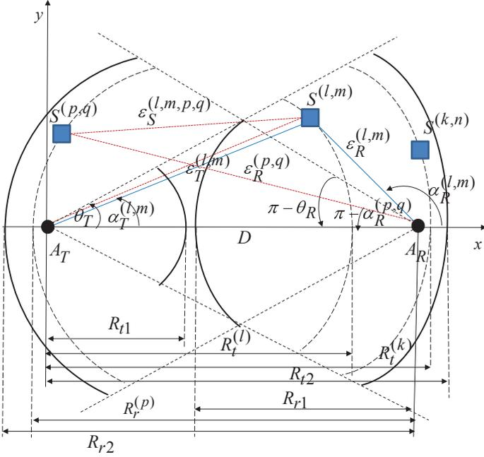
Fig. 1. The concentric-sectors model with LoS, SR, and DR rays for a wideband THz indoor channel.
