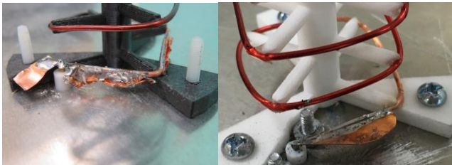
Fig. 10. Matching of the helix by a copper foil.
