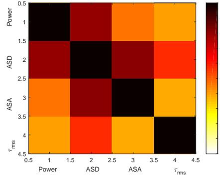
Fig. 4: Correlation coefficient matrix of specular parameters.
