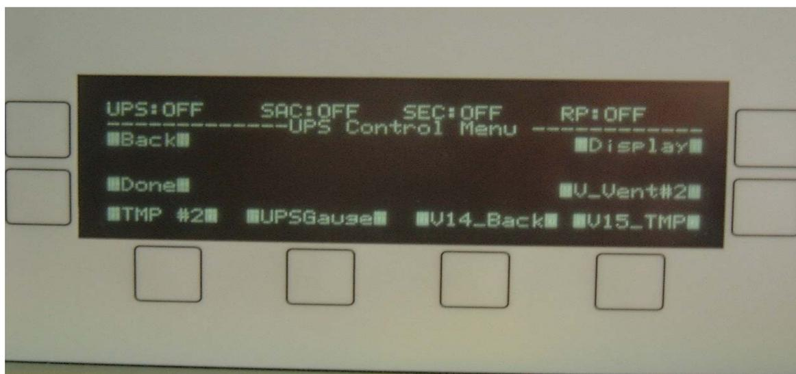
Figure 9. Vacuum control unit 'UPS control menu'
