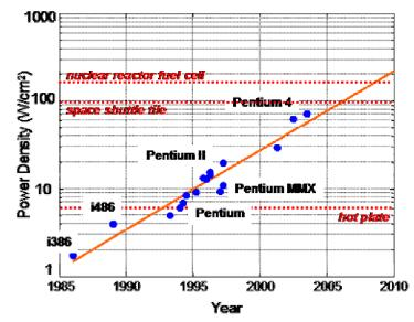
Figure 4. Power density of Intel microprocessor family Data from [14], [16]..
