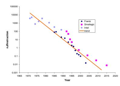
*Figure 3.* Energy per instruction for various processors. Data from [11],[12],[13].
