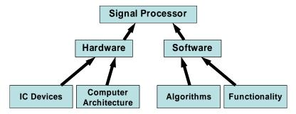
Figure 1. "Hardware" and "software" elements of a digital signal processor.
