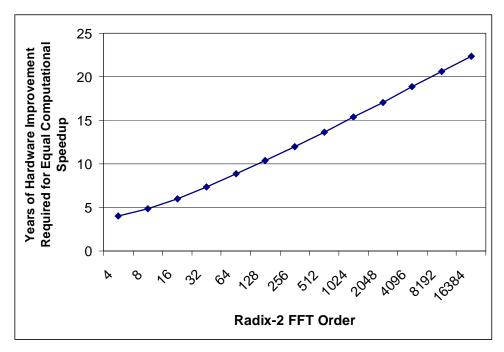
Figure 6. Years of Moore's Law improvement required to equal FFT computational savings relative to a sum-of-products DFT. Assumes hardware speedup of 1.5 orders of magnitude per decade (doubling every two years).
