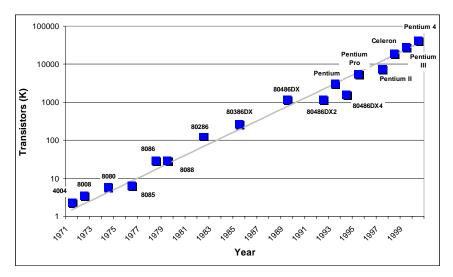
Figure 2. Growth in IC density as evidenced in Intel microprocessors. The solid line corresponds to an overall growth rate of 1.5 orders of magnitude per decade. Data from [9].
