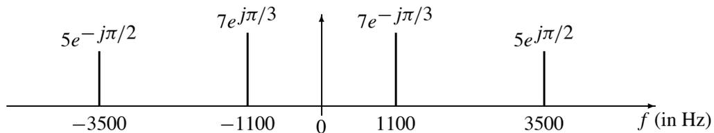
Determine the *discrete-time* spectrum for  $x[n]$  when  $f_{si} = 4000$  samples/sec. Make a plot for your answer, but label the frequency, amplitude and phase of each spectral component.
