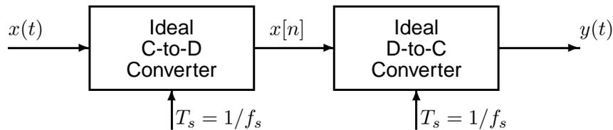
Figure 1: Ideal sampling and reconstruction system.
