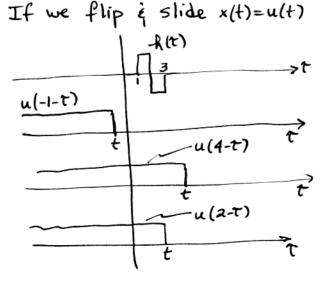
When t<1, there is NO overlap so y(t)=0 when t ≥ 3, there is complete overlap but the integral of h(r) is zero
