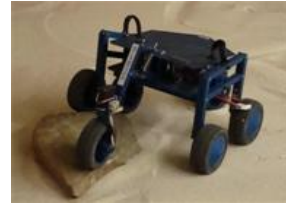
Fig. 7: SECT II (from Bluebotics, Inc.), rugged-terrain platform used for field survey.
