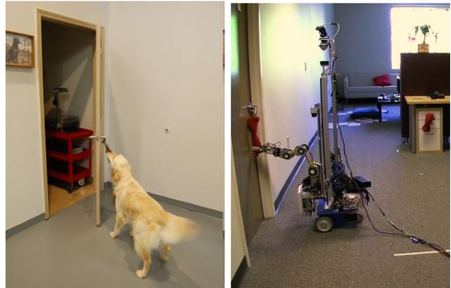
Fig. 1. On the left, a service dog opens a door using a bandanna tied to the door handle. On the right, our assistive robot opens a door in an analogous manner.
