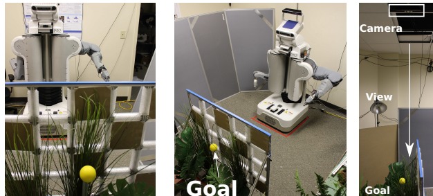
Fig. 1: Our method enabled a PR2 to select a base position, a torso height, an initial arm configuration, and an aperture to reach through in order to reach the yellow ball in the foliage. The label we used for this category of environment was foliage-aperture-clutter .
