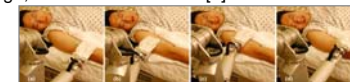
Fig. 14 Robot (a) wiping to left (b) to right (c) to left (d) completed
