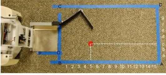
Fig. 5. Testing grasping area. Rectangle ABCD encircles the testing field. There are 7 markers on tape AD, and 15 markers on tape AB. The testing cylinder is placed on the mesh grids formed by these markers, e.g. the coordinate of cylinder shown in the figure is (5, c). Line BC and line OP are perpendicular to each other, and they define the starting position of the robot. The test is run with finger opened in the beginning.
