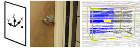
Fig. 3. Left: Coordinate axes parallel to the axes of the frame with the origin at the robot that is used by the door and door handle detection algorithms. Middle: Image of a door and handle. Right: The output of the door handle segmentation algorithm. The volume of interest (VOI) is the yellow box, the door is blue, the door handle is yellow, and the points inside the VOI are dark grey. The point cloud outside the VOI is light grey.
