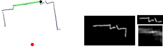
Fig. 5. Left: Position of the robot (red circle), the points from the laser scan (dark blue), the estimate of the door (green line) and the tracked position of the door handle (black circle) during the servoing behavior. Right: (clockwise from the left) Laser scan rotated and converted into an image, the template of the door handle and the result of correlation of the template with the image.
