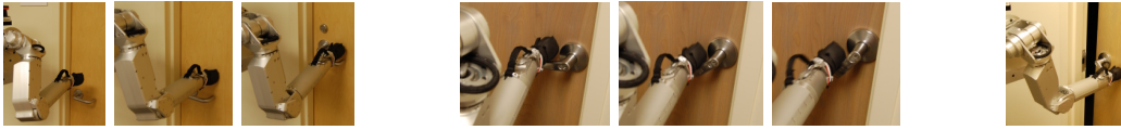
Fig. 6. Left: The robot reaches out to haptically detect the surface of the door and then moves down until it makes contact with the handle near the tip. Middle: The robot twists the handle. Right: The robot pushes open the door.
