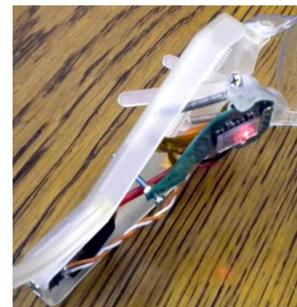
Fig. 9. A close-up of the more advanced wouse design, including springs and levers for adjusting the sensor position, battery (bottom left), and micro-USB charging receptacle (bottom left).
